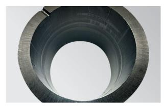
Typical debeaded pipe surface using the ClearBore tool.
